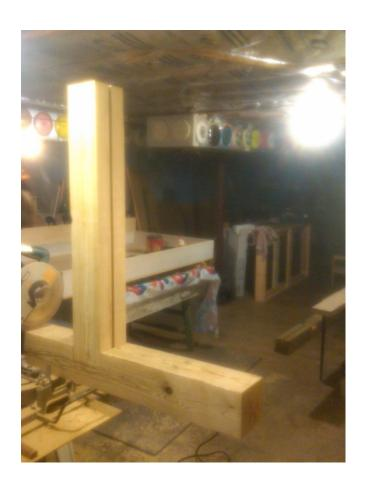
Once you get one notch cut, do a dry fit to make sure your notch is the right width for the cross board to fit perfectly. You may need to make some alterations.
