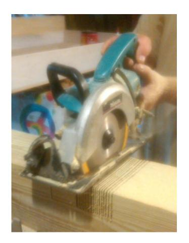
Use a skill saw to cut out your notches. Set the saw blade to 2" deep. Run several parallel cuts (20 or more) through the notch section.
