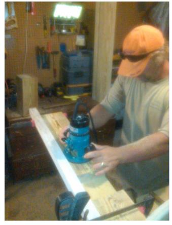
Once your notches are cut, you can route the channel out for the sign. Use clamps to clamp a guide to the **front edge** of the board. **Use the front edge for all three boards so that the channels line up.** Route from the top of the board toward the channel. It will take several passes at increasing depths to get all the material out of the channel. (1" router bit). The channel should be 1/2" deep.
