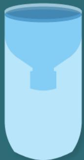
3 Draw inch marks on a piece of tape. Put rocks in bottom and fill with water to the "0" mark.
